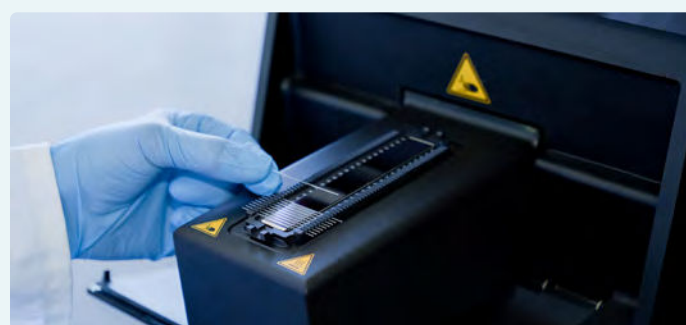
Figure 4. Easy sample introduction with capillaries.
