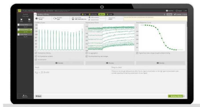
Figure 2. Dose Response Curve: The Dose Response analysis displays concentration-dependent changes of Ratio 670/650 nm, which are used to calculate K_d or EC50 values. The signal of each capillary is plotted against the ligand concentration in the capillary.
