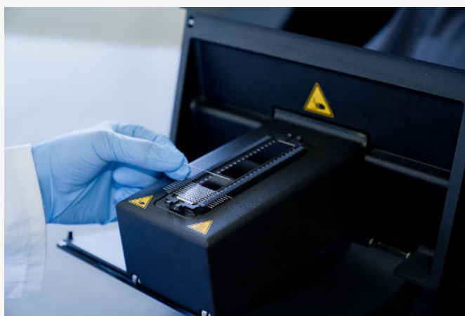
Figure 4. Easy sample introduction with capillaries.
