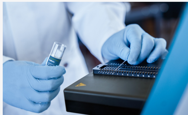
Figure 3. Easy sample introduction with capillaries.
